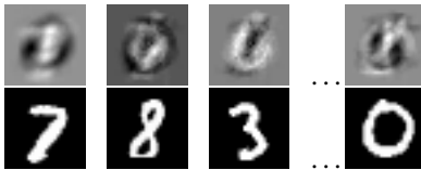
Figure 3: Bottom: A real mini-batch consisting of 100 examples from MNIST. Top: A forged mini-batch with verification error \epsilon \approx 2.5 \times 10^{-8} . We observe that the forged batches we generate consist of training examples from the original batch, but superimposed on top of each other. For logistic regression models, aggregation order changes result in errors on the order of 10^{-8} . See Appendix A.3 for details.
