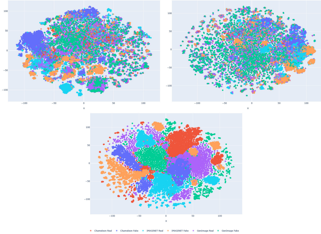
Figure 3: T-SNE Maaten & Hinton (2008) projection of GenImage Zhu et al. (2024), ImagiNet Boychev & Cholakov (2024), and Chameleon Yan et al. (2024) dataset. The CLIP+DINO (bottom) encoder successfully separates real and fake classes for each dataset unlike the other two options. (Top left: CLIP, Top right: DINOv2)
