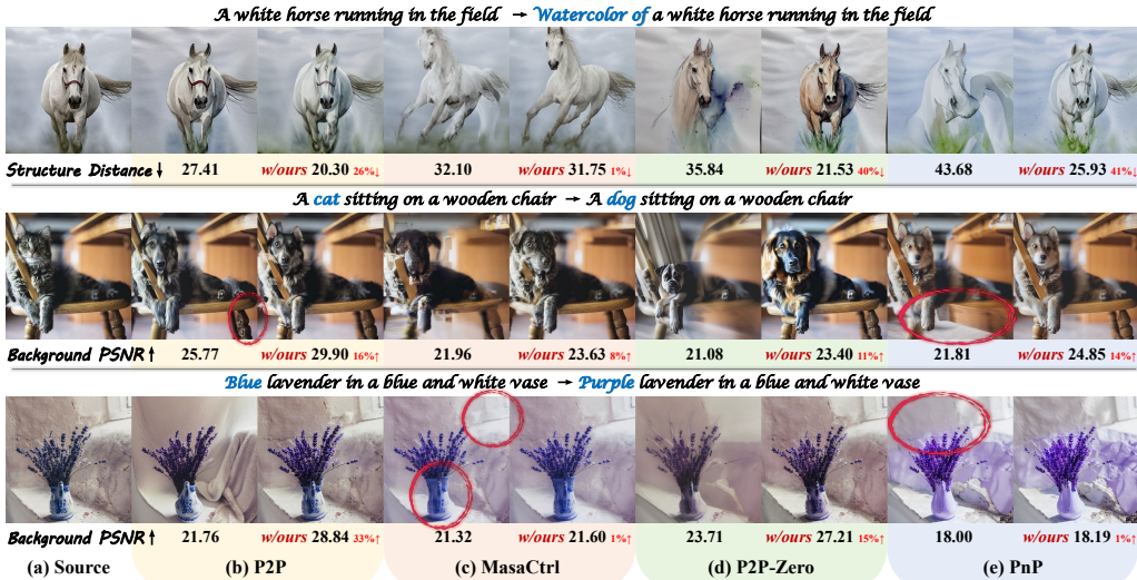
Figure 1: Performance enhancement of incorporating PnP Inversion into four diffusion-based editing methods across various editing categories (from top to bottom): style transfer, object replacement, and color change. The editing prompt is displayed at the top of each row, which includes (a) the source image, the editing results of (b) Prompt-to-Prompt (P2P) (Hertz et al., 2023), (c) MasaCtrl (Cao et al., 2023), (d) pix2pix-zero (Parmar et al., 2023), and (e) plug-and-play (Tumanyan et al., 2023). Each set of results is presented: the first column w/o PnP Inversion (Null-text inversion for P2P, DDIM Inversion for the others), and the second column w/ PnP Inversion . Incorporating PnP Inversion into diffusion-based editing methods results in improved image structure preservation (enhancement of the structure distance metric) for full image editing and enhanced background preservation (increased PSNR metric values in the background, i.e., areas that should remain unedited) for foreground editing. The improvements are mostly tangible, and we circle some of the subtle discrepancies w/o PnP Inversion in red. Best viewed with zoom in.
