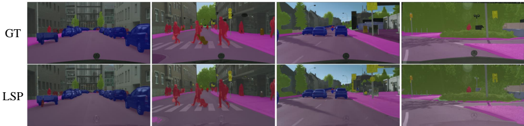
Figure 6: Qualitative result of segmentation masks on Cityscapes validation set predicted by SETR Zheng et al. (2021) with DeiT-Base/384 backbone remaining 50% FLOPs. First row shows ground truth mask and second row shows the predicted masks of pruned model.
