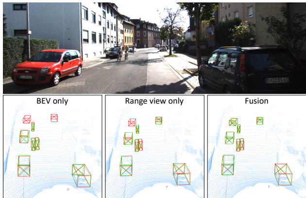
Figure 1: An example of detection results (in green) from BEV only, range view only, and attentive cross-view fusion settings, compared with ground truth (in red). Our attentive cross-view fusion of BEV and range view features could recall those distant objects with few points.
