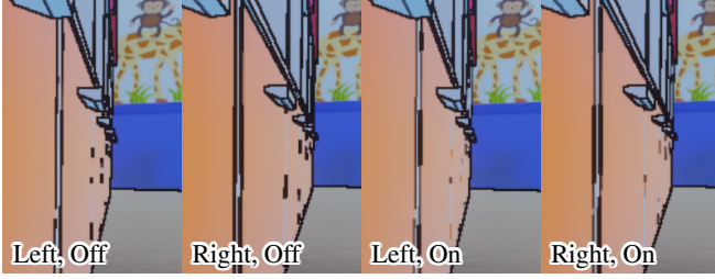
Fig. 7: Suppression of stereo-incoherent noise using reprojection and aliasing reduction. TAA is disabled to accentuate the effect.
