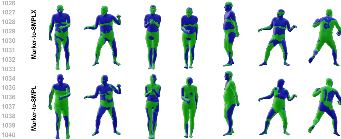
Figure 12: Visualizations of Marker-to-SMPLX and Marker-to-SMPL Regressors’ Performance. We display both the ground truth body mesh (in green) and the regressed body mesh (in blue). The greater the overlap between these two meshes, the better the regressor’s performance.
