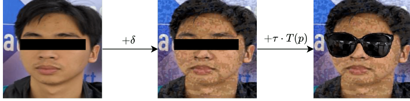
Figure 8: Procedure of LC attack in Facial Recognition. We add the adversarial perturbations to the poison instance before inserting the trigger into the appropriate facial area.
