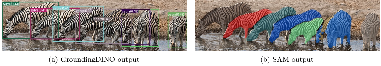
Figure 22: Illustration of the target segmentation step of LVLM-Count for the zebra image. The goal is to produce all the instance masks for E set to “zebra”. The cropped image from Figure 21, together with E , is given as input to GroundingDINO, which produces the output shown in Figure 22a. Figure 22a is then given as input to SAM, which produces the output shown in Figure 22b.
