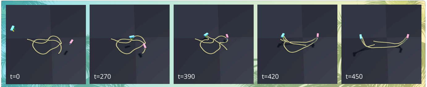
Fig. 1: Open-loop rollout of the particle-based ACT policy on an overhand-knotted rope excluded from the training set where t indexes simulation frames at 30 Hz. The policy predicts a single macro action (grasp and pull) from the initial particle state at t=0 ; for overhand knot configurations like the one shown, a single well-placed pull is sufficient to fully resolve the knot. The policy successfully transfers this strategy to some unseen rope instances.
