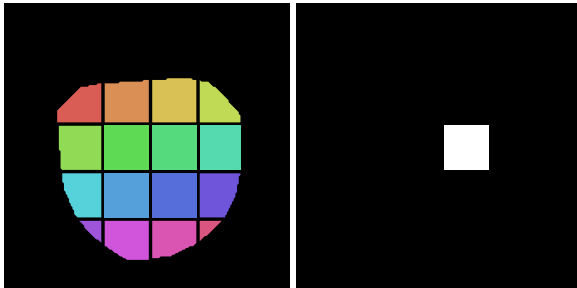
Figure 4: Left: illustration of the 4 \times 4 grid scheme, where the face is divided into a grid of 16 cells (each cell is denoted by a different color). Right: The mask M_{\tilde{y}_{loc}} is obtain by setting 1 to the pixels having the same color as the cell at position \tilde{y}_{loc} and 0 otherwise, in this case \tilde{y}_{loc} = 7 .
