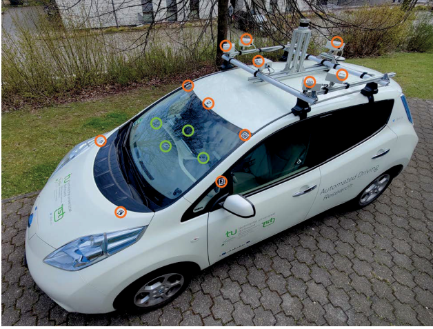
(a) Markers attached to the interior (circled green) and exterior (circled orange) of the test vehicle. Further markers are attached to the bottom of the lidar baseplate, behind the front camera and in the interior.
