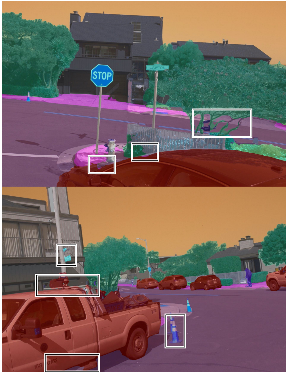
Figure 13: For the semantic segmentation mask predicted by SegFormer Xie et al. (2021) in original full resolution, some noise exists at the boundaries between regions with different semantic tags. These failure cases are more likely to occur at the corners of small objects.
