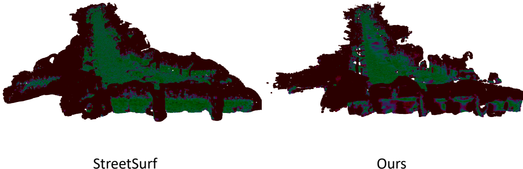
Figure 12: Illustration of the "before unveiled" geometry comparison with StreetSurf Guo et al. (2023). "Green" indicates "more accurate" regions, while "Red" represents "less accurate" regions. We empirically observe that the StreetSurf achieves higher accuracy on the observable ground of the street. Even after fair mesh cropping, the reconstructed mesh of StreetSurf is still influenced by out-of-range meshes to some extent. This effect stems from inherent methodological differences between SDF extraction and TSDF fusion, which may contribute to a slightly lower F-Score for the SDF extraction approach. Overall, the reconstruction performances are comparable.
