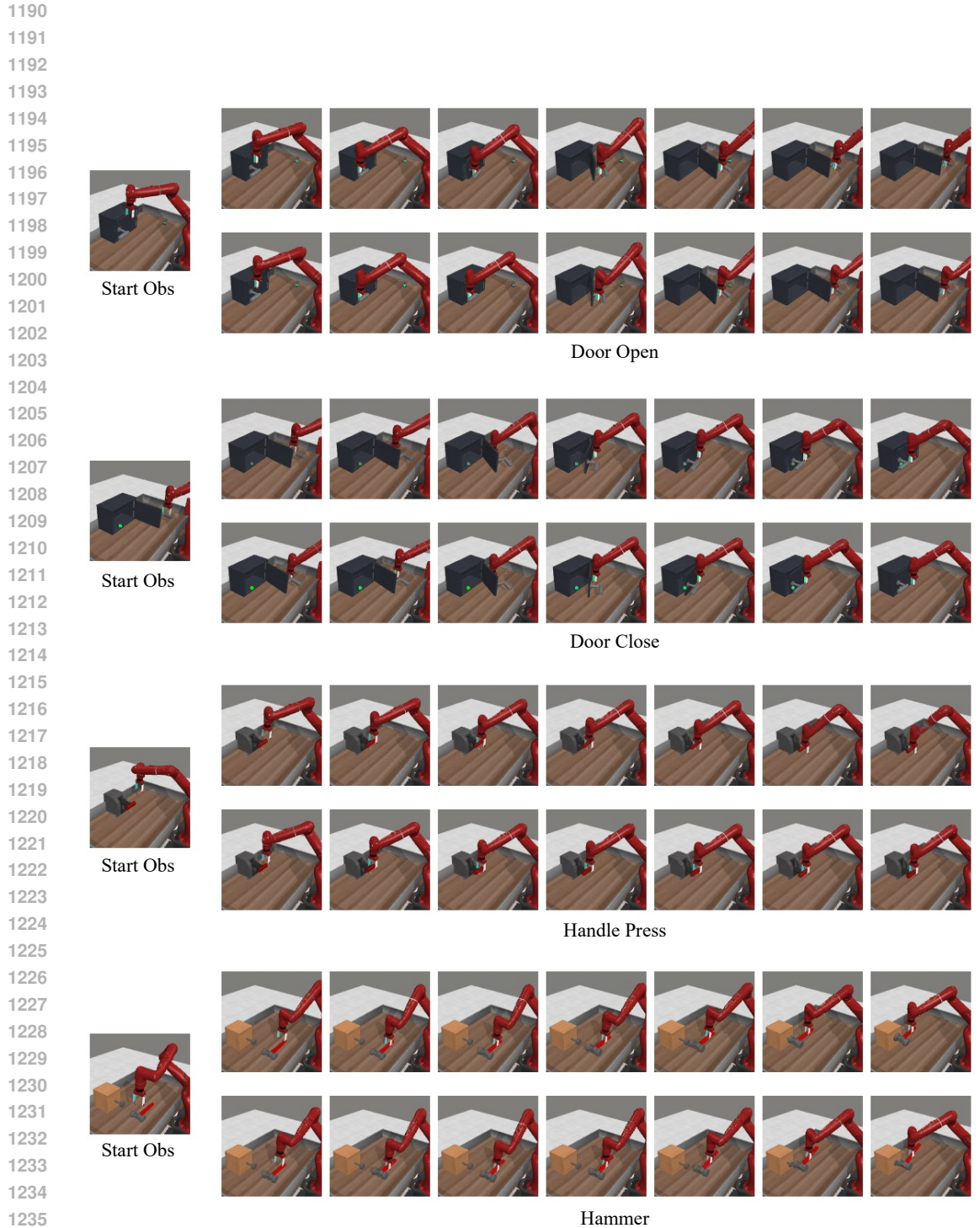
1237 1238 1239 1240 1241 Figure 12: Additional Qualitative Results of the Generated Videos and Our Policy Rollout of 4 tasks on Meta-World. We present qualitative results of four tasks in Meta-World Environment. For each task, results are displayed in 2 rows: the first row of images are the generated video from the video model conditioned on the start observation image and task description, and the second row of images are the rollout of our policy conditioned on the corresponding frames from the generated video. The task prompts provided to the video model are shown below the respective images.
