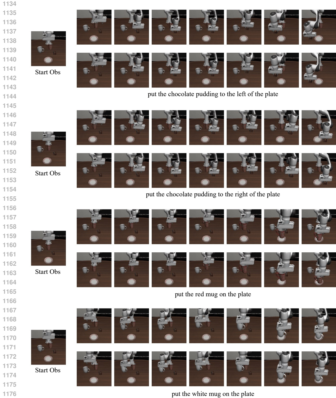
Figure 11: Additional Qualitative Results of the Generated Videos and Our Policy Rollout on Libero Scene 2. We present qualitative results of four tasks in Libero Scene 2. For each task, results are displayed in 2 rows: the first row of images are the generated video from the video model conditioned on the start observation image and task description, and the second row of images are the rollout of our policy conditioned on the corresponding frames from the generated video. The task description provided to the video model are shown below the respective images.
