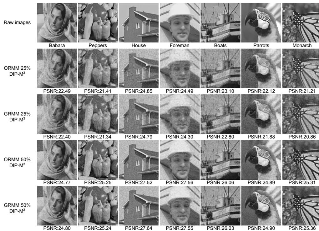
Figure 12: Qualitative comparison on different measurement matrix with 50 looks on RMM task. The first row shows the raw test images. The second and third row are RMM (25% sampling rate) with random orthogonal and Gaussian measurement matrix. The fourth and fifth row are RMM (50% sampling rate) with random orthogonal and Gaussian measurement matrix.
