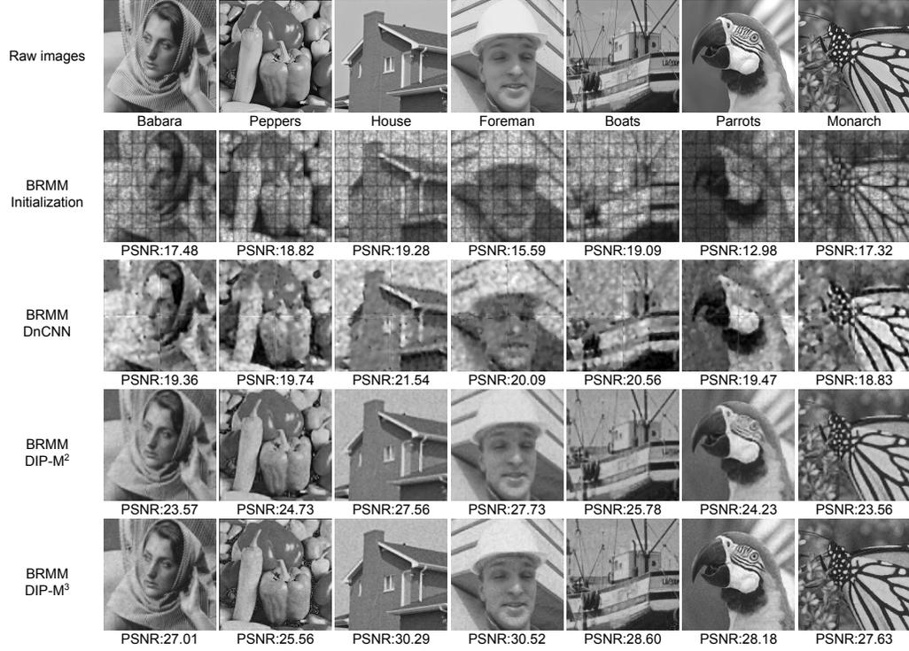
Figure 7: Qualitative comparison on BRMM with 50 looks. The second row visualize the initialization  $\frac{1}{L} \sum_{l=1}^L |y_l|$ , which is the same for all models. From the third row to the last row, we show the reconstructed results from DnCNN, DIP-M<sup>2</sup> and DIP-M<sup>3</sup> respectively.
