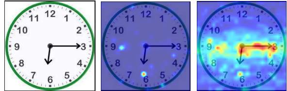
Figure 1: Our proposed PlaM improves visual grounding and prediction. Given the clock image (left) and the question "It is ( ) past six.", the original MLLM without PlaM attends diffusely and answers "half" (middle). After applying PlaM model merging, attention concentrates on the clock hands and the model correctly answers "quarter" (right).
