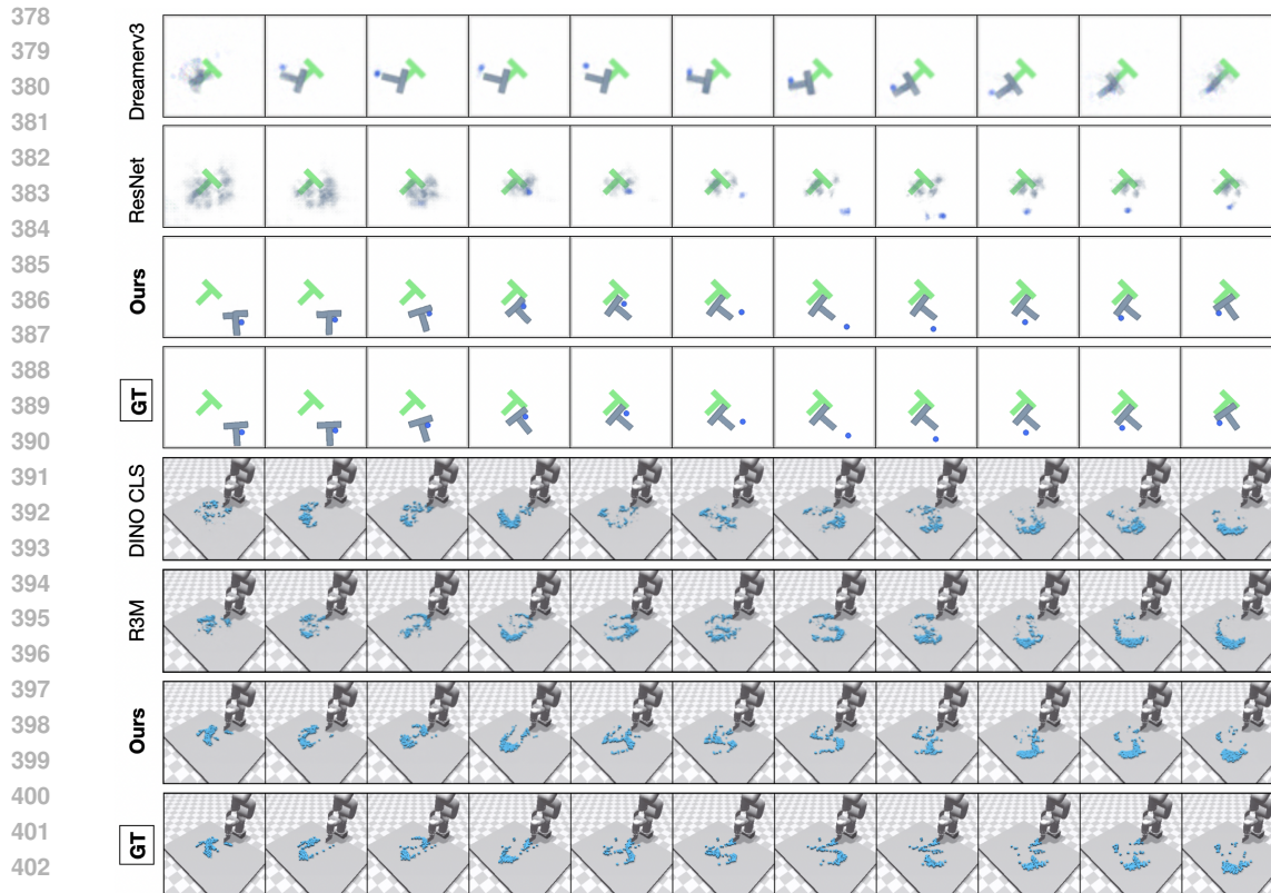
Figure 4: Openloop rollout of world models trained with various pre-trained encoders on Push-T and Granular environment. For each trajectory, the model is given the first frame as well as sequence of actions. The world models performs openloop rollout with these actions, and the images are reconstructed by a pre-trained decoder. For each environment, the bottom row denotes the ground truth. DINO-WM (Ours) rollouts are bolded and are visually indistinguishable from the ground truth observations.
