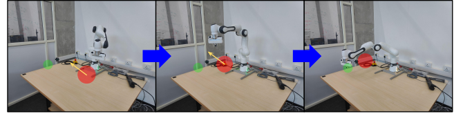
Fig. 4: Illustration shows Franka Panda manipulator advancing toward its designated target ( green region ) while executing collision avoidance maneuvers in the presence of a dynamic obstacle ( red sphere ). Arrows indicate direction.
