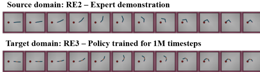
Figure 29: (Top) An example trajectory of image observations generated by \pi_E in the source domain. (Bottom) An example trajectory of image observations generated by \pi_\theta trained using D3IL for 1 million timesteps in the target domain.
