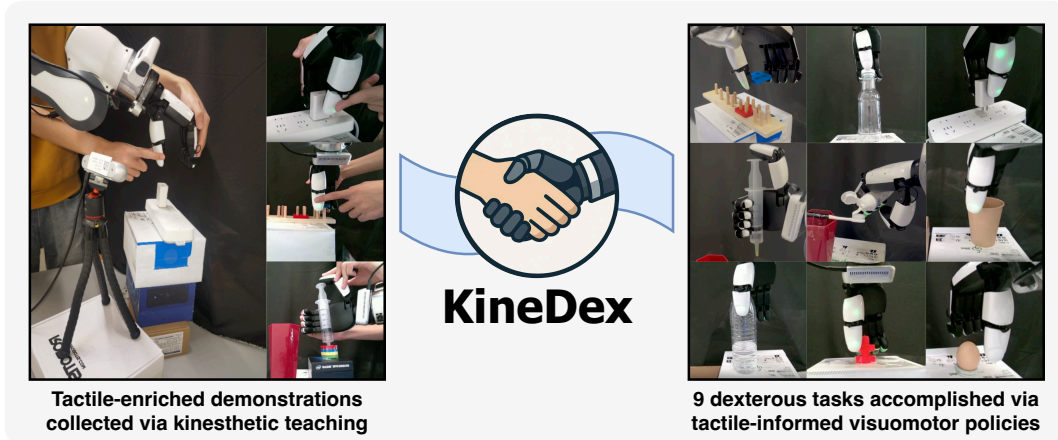
Figure 1: We present KineDex , a framework for collecting tactile-enriched demonstrations via kinesthetic teaching and training tactile-informed visuomotor policies for dexterous manipulation.
