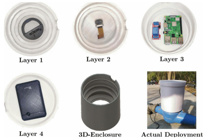
Figure 3: 3D structure and deployed model
