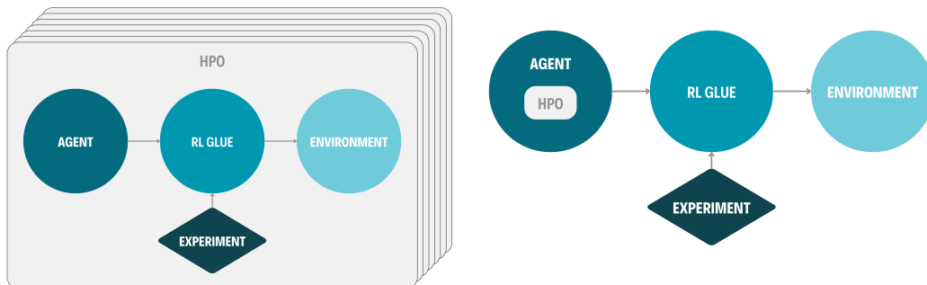
Figure 1: Contrasting the typical hidden tuning setting (left) versus the proposed online tuning setting (right). The online tuning setting requires that tuning is a part of the agent, as it must tune the hyperparameters online, during interaction. Hidden tuning layers optimize the hyperparameters outside of the agent-environment interaction, allowing a separate search to be performed.
