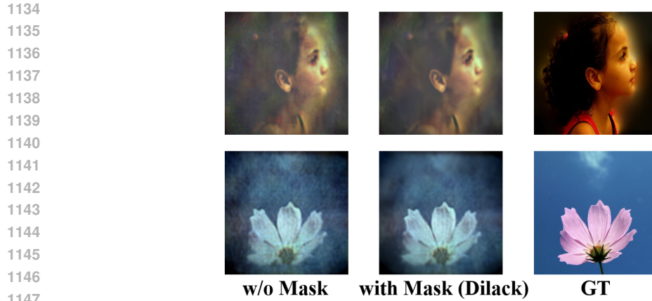
1148 Figure S3: The qualitative comparisons for the effectiveness of the ROI mask in ‘real’ lensless 1149 camera dataset. ‘w/o Mask’ refers to s_\theta + \mathcal{L}_{\text{PiAC}} , while ‘with Mask’, which is Dilack, refers to 1150 s_\theta + \mathcal{M}_{\text{ROI}}[\mathcal{L}_{\text{PiAC}}] . 1151
