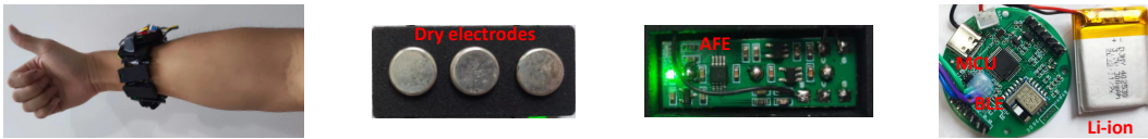
Figure 11: In-house developed sEMG acquisition system: from left to right are the acquisition system, dry electrodes, AFE, MCU with BLE 5.2 module, respectively.
