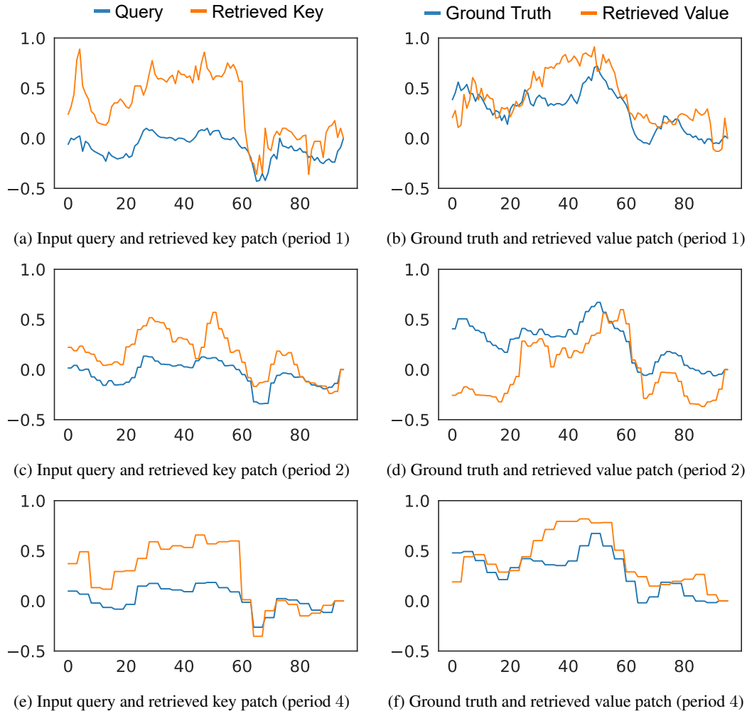
Figure 7: The example of our retrieval results on ETTh1 dataset. The key patches retrieved by period 1, 2, and 4 are compared with input query in (a), (c), and (e), respectively. The value patches retrieved by period 1, 2, and 4 are compared with ground truth in (b), (d), and (f), respectively. Note that the figures in the right side sequentially follows after the figures in the left side within the time series.
