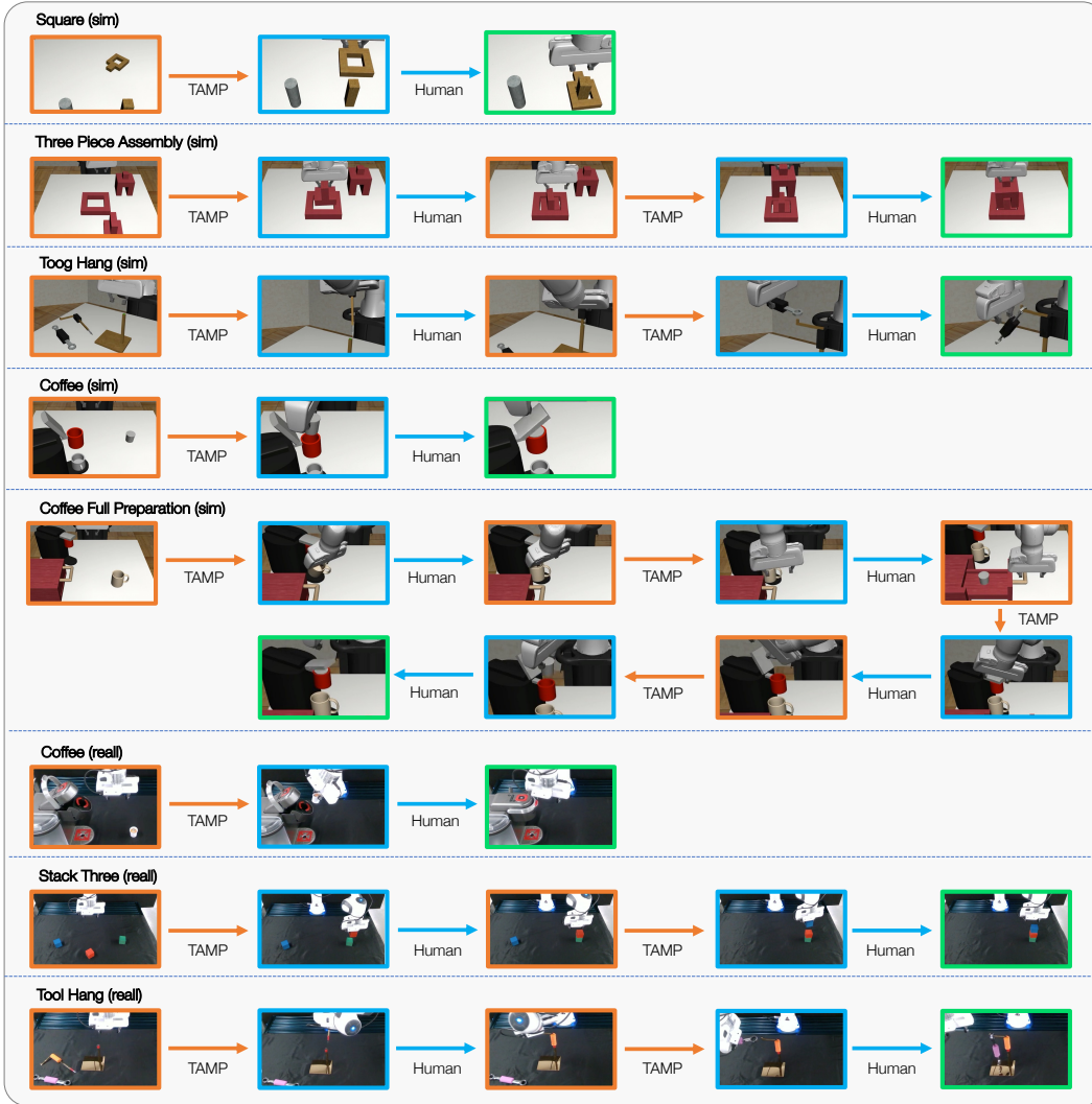
Figure E.1: Task Segments. We show the human and TAMP segments for each task.
