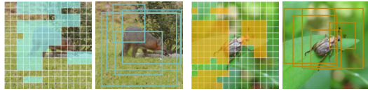
Figure 2: Illustration of random block-wise sampling and random cropping. Random block-wise sampling is used in our approach. Random cropping is a key data-augmentation scheme for contrastive pretraining.
