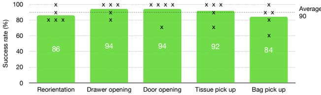
Fig. 4: Success rate of Robot Utility Models on average over five novel scenes in five different tasks, with automated retrying in each trial. The X’s on the figure denote success rates from individual environments.
