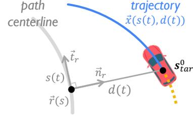
Figure 2: Trajectory generation in a Frenét Frame
