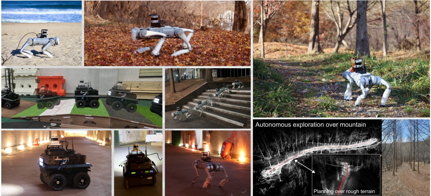
Fig. 1: Point Navigation Transformer (PointNT) is a sequential transformer-based navigation policy equipped with a powerful 3D point cloud encoder, designed for navigation and exploration in diverse and challenging environments. We evaluate PointNT in both real-world and simulation settings, deploying it on two different robotic platforms (legged and wheeled) in real-world experiments, and three platforms (legged-wheel, wheeled, and tracked) in simulation, all using a same transformer policy, which showcase our ability of proposed approach.
