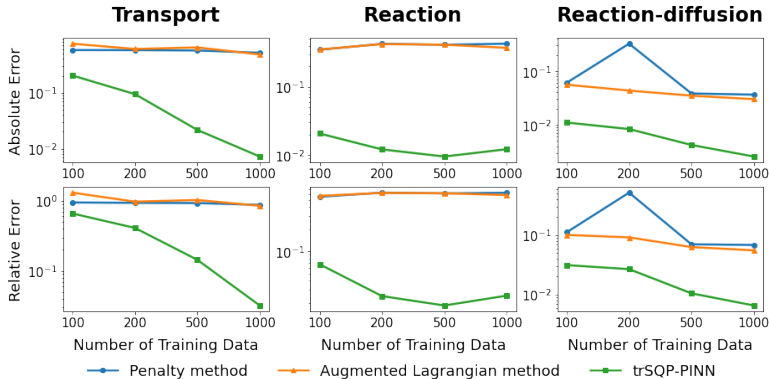
Figure 3: Absolute and relative errors of three hard-constrained methods with varying number of training data points. TrSQP-PINN consistently outperforms the other methods and maintains low errors even if it is trained on a small dataset.
