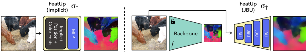
Figure 4: Our Implicit version of FeatUp learns an implicit network to upsample a single image’s features. Our JBU FeatUp learns a stack of JBUs that learns to quickly upsample features from a large image corpora.
