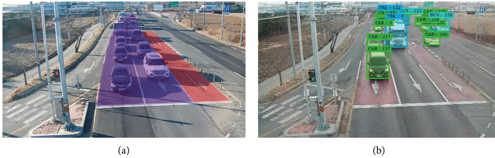
FIGURE 6: Result of object detection of smart intersection. (a) Region of interest (RoI) setting. (b) AI model inference for object detection.
