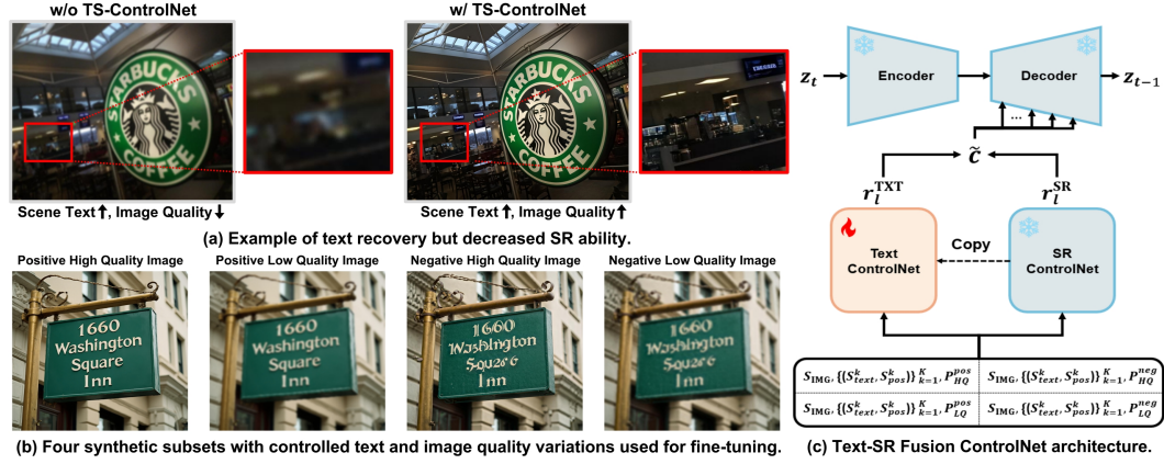
Figure 3: Text-centric fine-tuning framework: (a) trade-off between scene-text fidelity and overall image quality according to guidance; (b) four synthetic training subsets with matched prompts; (c) TS-ControlNet architecture.
