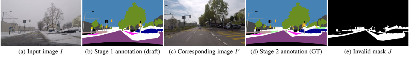
Fig. 2. Illustration of semantic annotation protocol for ACDC. The color coding of the semantic classes matches Fig. 1. All annotations in (b), (d) and (e) pertain to the input image I in (a). A white color in (b) and (d) denotes unlabeled pixels.
