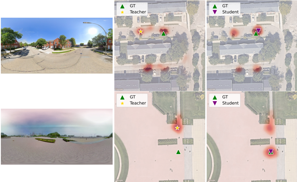
Figure 3: CCVPE teacher and student model’s predictions on VIGOR test set. The red color denotes the localization probability (a darker color means a higher probability).
