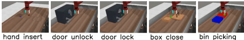
Figure 4: For each task in the Meta-Learning 45 (ML45) benchmark in the MetaWorld environment, we use a scripted policy to collect a diverse dataset of robot behavior. We use the demonstrations from the 45 training tasks to pretrain our Transformer policy. We then train separate adapters for each test task (shown in the Figure) through imitation learning using the respective demonstrations. Object and goal positions are randomized at the start of every episode during data collection and inference time.
