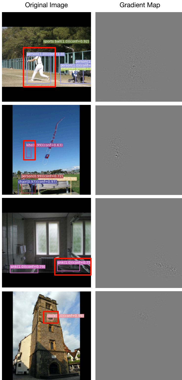
Figure 5: Left : detection results for original image; Red BBox : the target object from which we back-prop gradients; Right : the gradient flowing from the object bounded by red bounding box. Pixel values are normalized using the min-max rule.
