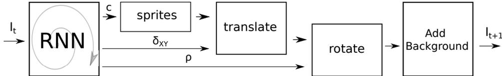
Figure 2: A schematic block diagram for a Perception Updating Network. This configuration uses both convolutions with delta functions for translation and spatial transformers for rotation. It also shows the optional background underlay.
