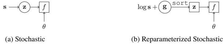
Figure 3: Stochastic computation graphs with stochastic nodes corresponding to permutations. Squares denote deterministic nodes and circles denote stochastic nodes.
