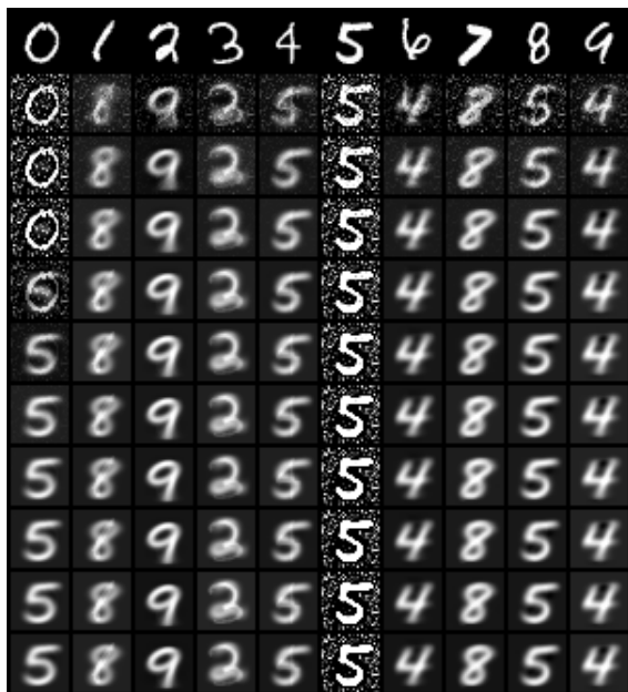
Figure 13: Perturbed images at the end of 100-step PGD attack using (untargeted) C&W approximation. The 11 rows show the images after 0, 10, 20, ..., 100 steps of PGD.
