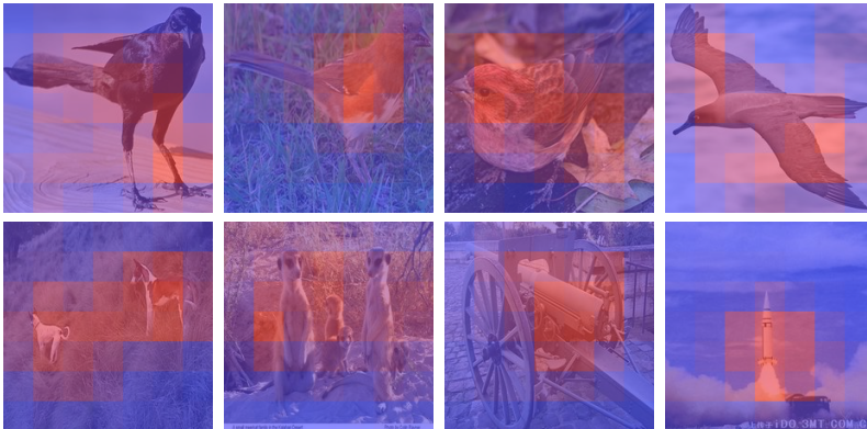
Figure 1: Examples of images from CUB (top) and miniImageNet (bottom) overlaid with entropy-based spatial attention maps obtained from (8) using only the predicted class probabilities from ResNet-18 pre-trained on Places. See section 5 for details on datasets and networks.
