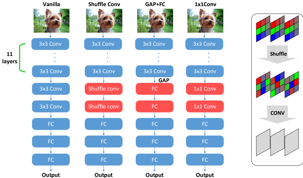
Figure 1: Left: A demonstration of Shuffle Conv , GAP+FC and 1x1Conv on a VGG-16 architecture, where last 2 conv layers are modified accordingly. Right: The detail of the shuffle conv . Each feature map from the input tensor will be randomly and independently shuffled before being fed into an ordinary convolution.
