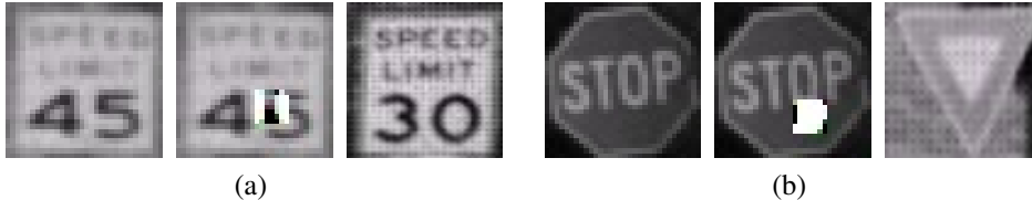
Figure 7: Examples of the ROA attack on traffic sign, using a rectangle of size 7 \times 7 . (a) Left: the original Speedlimit45 sign. Middle: modified input image (ROA superimposed on the sign). Right: an image of the predicted which is Speedlimit30 with the adversarial input in the middle image. (b) Left: the original Stop sign. Middle: modified input image (ROA superimposed on the sign). Right: an image of the predicted Yield sign with the adversarial input in the middle image.
