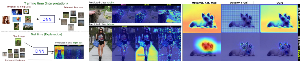
Figure 1: Left: Proposed training/testing pipeline. Center: Visual explanations generated by our method. Predicted class labels are enriched with heatmaps indicating the pixel locations, associated to the features, that contributed to the prediction. Note these features may come from the object itself as well as from the context. On top of each heatmap we indicate the number of the layer where the features come from. The layer type is color-coded (green for convolutional and pink for fully connected). Right: Visualization comparison. Note how our heatmaps attenuate the grid-like artifacts introduced by deconvnet-based methods at lower layers. At the same time, our method is able to produce a more detailed visual feedback than up-scaled activation maps.
