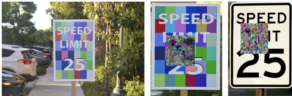
Figure 1: Redesigned speed limit sign (left) with attacks on redesigned (middle) and original (right).
