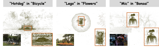
Figure 4: Visualization of the point cloud produced by our SecureGS without region-aware density optimization (RDO) strategy. The RGB reference of the hidden scene is placed on the left bottom.
