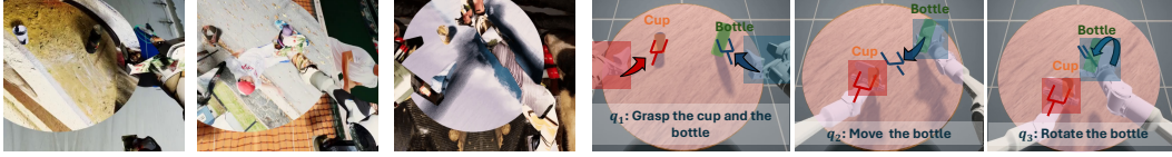
Figure 3: An example of the DR flow (left three images) and the chain of affordances (right three images) generated in the simulated environment for the water-pouring task.
