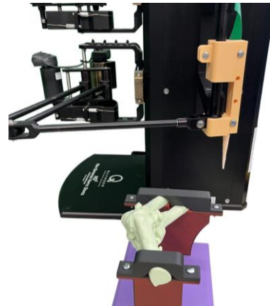
Fig 1. Quanser HD2 with custom single-tip probe and 3D-printed elbow phantom mounted on a rigid holder.
