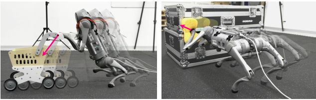
Fig. 4: Snapshots of two whole-body loco-manipulation tasks, where the desired EE force are overlaid as pink arrows. Upper : pushing a shopping cart while walking in bipedal mode; bottom : holding a sponge while walking in quadrupedal mode.
